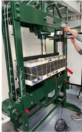
Figure 4.17: The TES heat exchanger in the hydraulic press apparatus
