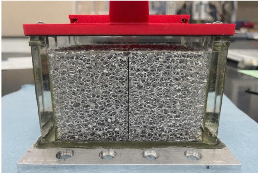
Figure 7: Metal foam test section composed of two Duocell metal foam block and a similar PCM containment method.
